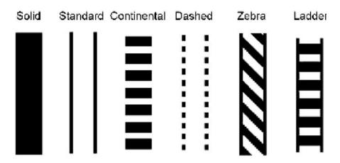
**EXHIBIT V-24**Example of Crosswalk Marking Patterns (Note: Neither the solid crosswalk nor the dashed lines (which are common in Europe) are included in the 2000 MUTCD.)
