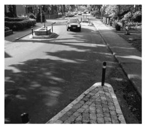
**EXHIBIT V-40**A chicane consists of alternatively placed curb extensions into the street which creates a horizontal shift in traffic and reduced vehicle speeds. (Photo by Dan Burden)
